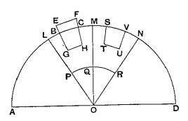
Then, since the pressure on the parts of the fluid at PQ, QR must be equal in order that the fluid may be at rest, it follows that the weight of the portion STUV of the fluid must be equal to the weight of the solid EGHF. And the former is equal to the weight of the fluid displaced by the immersed portion of the solid BGHC.
