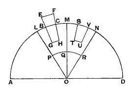
Conceive also another pyramid in the fluid with vertex O, continuous with the former pyramid and equal and similar to it. Let the pyramid so described be cut in OM, ON by the plane of ABCD.
