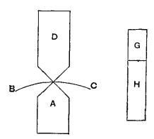
Therefore the weight of the fluid displaced is (G+H), and hence the volume of the fluid displaced is the volume of the solid A. There will accordingly be rest with A immersed and D projecting.
